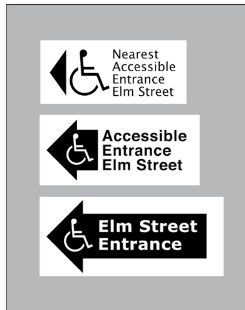
Examples of signs for inaccessible shelter entrances directing people to the accessible entrance.
